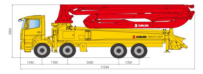
\* Remark: Standard specification with BENZ MB4141 Actros. Dimension depends on truck specification.
